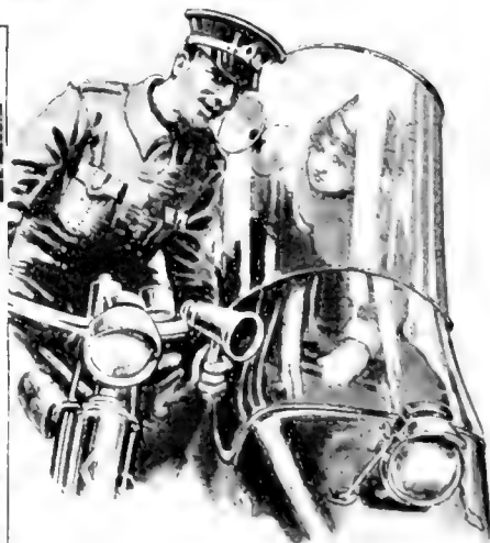
Above: A sidecar hood and windshield made of transparent material. A speaking trumpet facilitates communication with the driver of the car
